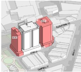
The upper most level of the tower (level 16) houses the rooftop terrace and presents as a recessed level that also houses plant rooms for fire/ mechanical etc. Above this a, lightweight steel 'pergola' roof provides shading to the terrace area.
